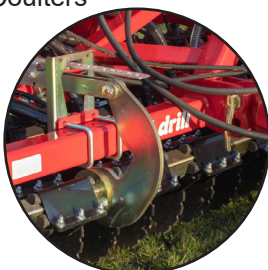
Hydraulic Adjustable Coulters
