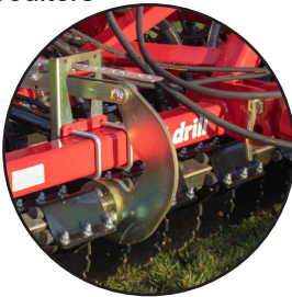
Hydraulic Adjustable Coulters
