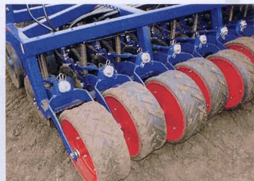
Light, moist soils were not a big test for our Moore DP600A Tandem Uni-drill. Nonetheless the 6m wide machine made an impressive job of accurately placing protein pea seed.
