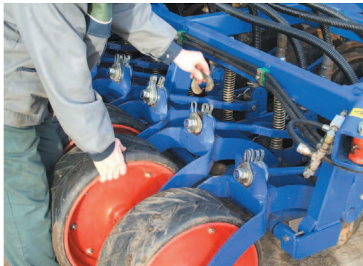
Adjusting the depth of the seed using spring clip spacers.
