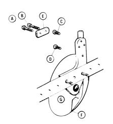
The leading edge of the seed coulter should be set parallel to the disc and just touching it. This can be achieved by means of the retaining bolts A and B and the adjusting screws C and D. If the tip, F, of the seed coulter is out from the disc, this can be corrected by tightening bolt A (front bolt) more than bolt B, while the top, G of the seed coulter can be brought in towards the disc by tightening Bolt B (rear bolt) more than Bolt A.
