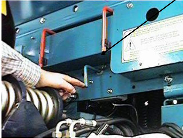
The seed box can be very easily cleaned out, by pulling the two red levers, which will empty the seed box via two tubes. This is best done when the machine is folded and fully lowered on the ground.
