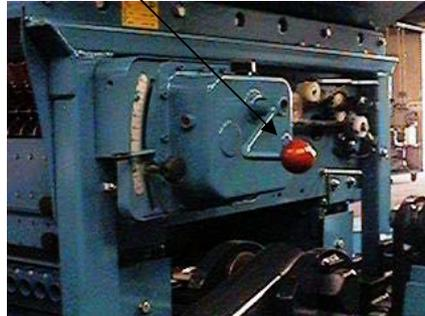
6. Turn handle the required number of turns for the width of drill according to the chart below.
