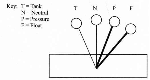
Failure to disengage the fan through the float facility on the spool lever, will 'dead head' the hydraulic motor, this may then destroy the manometer or damage the fan motor seals.
