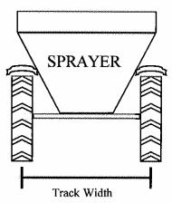
The above measurement can then be used to determine the coulters on each side of the drill that will allow a tramline track width approximately equal to your sprayer track.
