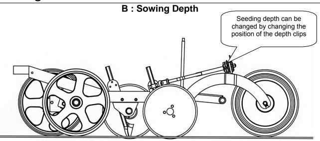
By moving depth clips from the 'A' side to the 'B' side and vise versa the seeding depth can be adjusted
