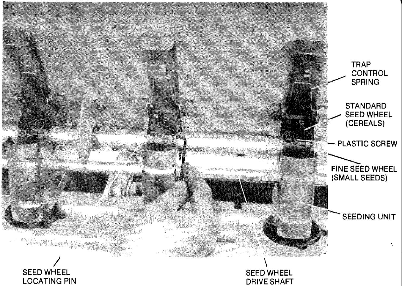
FIGURE 4. FEED TRAP POSITIONS
