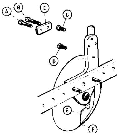
To obtain better depth control for small seeds e.g. oil seed, rape, turnips etc. in loose or cultivated soil it may be necessary to lower the tip of the seed tube coulters almost to the edge of disc.
