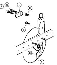
To obtain better depth control for small seeds e.g. oil seed, rape, turnips etc. in loose or cultivated soil it may be necessary to lower the tip of the seed tube coulter almost to the edge of disc.
