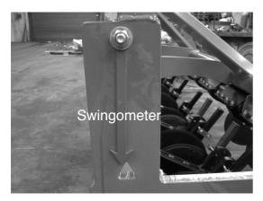
Set the tractors draft links in such a way that the seed drill can swing sideways only very slightly, and so that each arm can float independently, and allow the rear packer to control the seeding depth independently of the tractor. After hitching on to the lower links, raise the drill and fold up the parking stands, slide them inside the chassis and secure with the linch pins provided.
