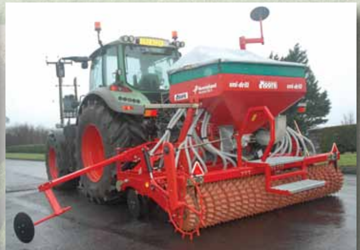
Mounted Unidrill with markers, tramliner and hopper extension.
