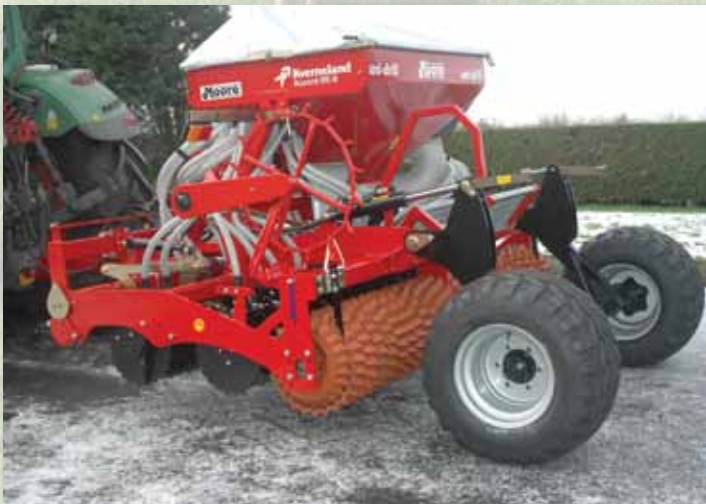
Trailed Unidrill with 480/45-17 floatation tyres and soft ride suspension
