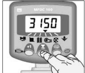
Figure 16: Display Fan Speed
