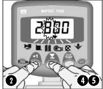
Figure 18: Set low speed alarm threshold
