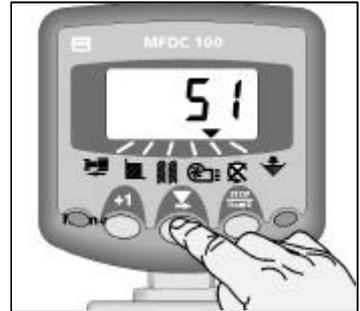
Figure 19: Distribution Shaft speed
