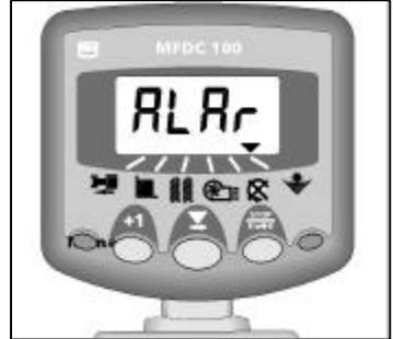
Figure 20: Hopper Low Alarm
