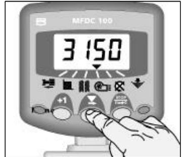
Figure 16: Display Fan Speed
