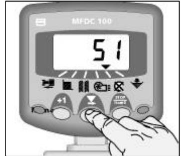
Figure 19: Distribution Shaft speed
