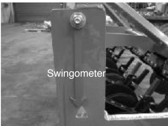
Set the tractors draft links in such a way that the seed drill can swing sideways only very slightly, and so that each arm can float independently, and allow the rear packer to control the seeding depth independently of the tractor. After hitching on to the lower links, raise the drill and fold up the parking stands, slide them inside the chassis and secure with the linch pins provided.
